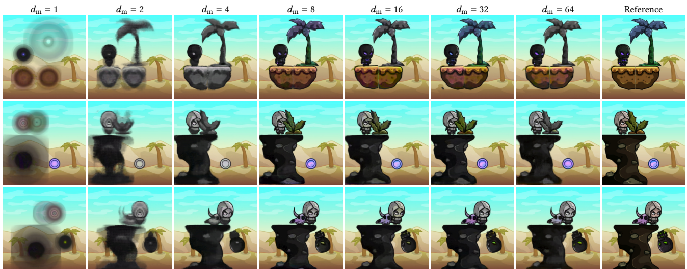
Fig. 2. Impact of the size d_m of the material representation on the quality of rendered results. The results with d_m = 32 feature highest quality; we used this configuration to generate all results in the main article and in the other figures in this supplementary document.
